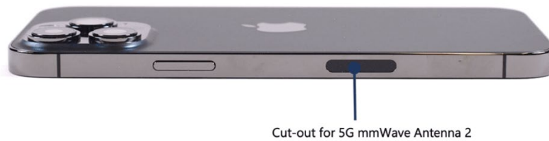
Figure 4. Exterior cut-out for iPhone 13 antenna. 58 The FCC nor the FDA feature information informing the public where antennas exist on their cell phones, nor recommend that the public avoid pointing those antennas at their eyes or skin.
